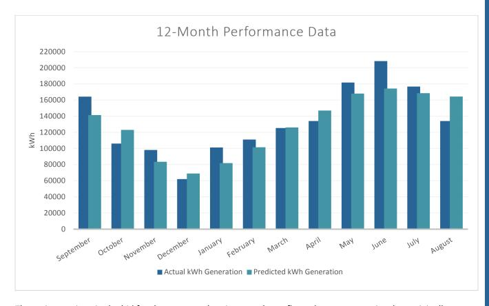
The estimate given in the bid for the system, when increased to reflect a larger system size than originally designed, claimed annual production would be about 1,547,582 kWh per year. The actual generation numbers from the Geneseo PV system are outproducing this estimate with 1,601,724 kWh generated between September 2015 and August 2016. The real-time generation data can be found <a href="here">here</a>.
