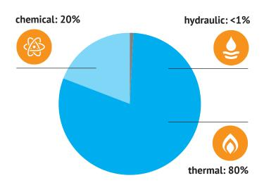
Wastewater contains nearly five times the amount of energy needed for the wastewater treatment process — the majority in the untapped area of thermal energy.
